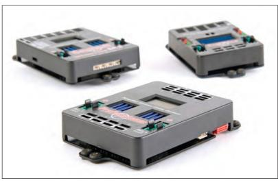
At around the size of a smartphone, most PowerBox units weigh between 100 and 200g.
