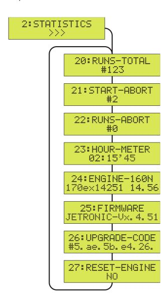
To quit the 2:STATISTICS menu and to return to the SETUP menu, press the SET key for more than 2 seconds (ESC).
