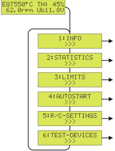
To enter the SETUP menu for configuring the firmware parameters, first press the SET key and then use the Up/Down keys to switch between the available parameter sections.
