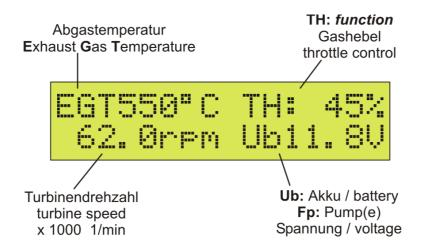
TH# = Throttle is a combined function display and error display for the engine operation.
