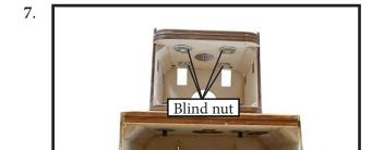
Attach the motor to the front of the electric motor box using four 4mm blind nut, four M4x20mm hex head bolts to secure the motor. Please see picture shown.
