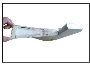
Slide the vertical stabilizer into the slot in the top of the fuselage. The rear edge of the stabilizer should be flsh with the rear edge of the fuselage and the lower rudder hinge should engage the precut hinge slot in the lower fuselage. The bottom edge of the stabilizer should also be fimly pushed against the top of the horizontal stabilizer.
