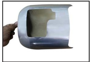
Tape the cowl to the fuselage using low-tack tape.
