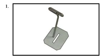
Remove each hinge from the wing panel and aileron and place a T-pin in the center of each hinge. Slide each hinge into the wing panel until the T-pin is snug against the wing panel. This will help ensure an equal amount of hinge is on either side of the hinge line when the aileron is mounted to the aileron.
