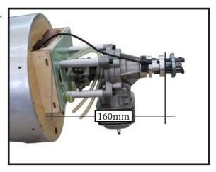
Position the engine with the drive washer (160mm) forward of the firewall.
