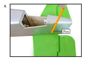
Remove the stabilizer. Using the lines you just drew as a guide, carefully remove the covering from between them using a modeling knife.
