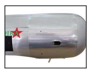
Install the muffler and muffler extension onto the engine and make the cutout in the cowl for muffler clearance. Connect the fuel and pressure lines to the carburetor, muffler and fuel filer valve. Secure the cowl to fuselage using the M3x10mm socket head screws. Putting a small length of silicon fuel tube under the head of the screw helps with vibration.
