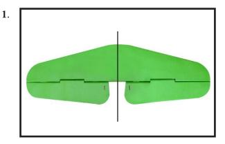
Using a modeling knife, carefully remove the covering at mounting slot of horizontal stabilizer (both side of fuselage).
