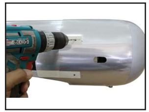
With the muffler, needle valve, and spark/ glow plug removed from the engine, slide the cowl in place over the engine. Temporarily install the propeller and spinner in order to fid the exact location of the cowl. When satisfied with the cowl placement, secure the cowl to the fuselage using masking tape.
