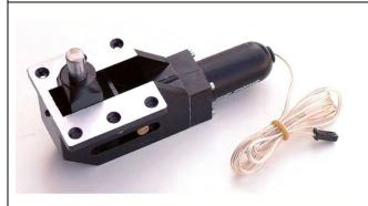
Art. CRA/15890/303 Giant Retractable Electric L/G travel 95° fixed Body and cam duralumin Wire length 1 mt.
