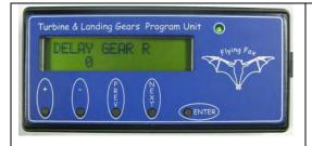
Press the "NEXT" key to enter the right electric landing gear "closure starting delay" programming page "DELAY GEAR R" This control is used in particular to adjust the landing gears closure in the "delay amongst themselves" mode as in the W.W.II fighting planes
