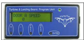
Press the "NEXT" key to enter the programming page in which it is possible to adjust the wheel doors group A servos' speed
