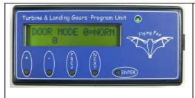
Press the "NEXT" key to enter the programming page in which it is possible to select the wheel doors A and B group working mode "DOOR MODE"
