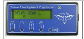
Press the "NEXT" key to enter the left electric landing gear "closure starting delay" programming page "DELAY GEAR L" This control is used in particular to adjust the landing gears closure in the "delay amongst themselves" mode as in the W.W.II fighting planes
