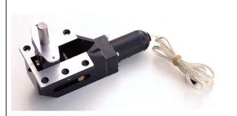
Art. CRA/15890/302 Giant Retractable Electric L/G travel 95° steerable Body and cam duralumin Wire length 1 mt.
