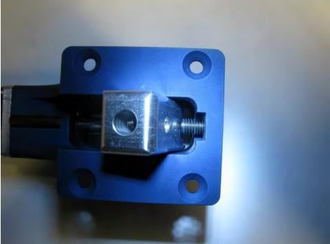
Screwing in the end-stroke screw too tightly could result in damage to the cam which will push strongly on the rim of the screw thereby preventing the sphere from working correctly
