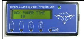
Press the "NEXT" key to enter the "maximum supplying power time" programming page "MAX POWER TIME"; this control was created as an additional safety measure to prevent the landing gears remaining locked open or close
