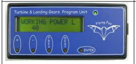
Press the "NEXT" key to enter the left landing gear (L) "working power supply" programming page "WORKING POWER L"
