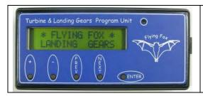
Plug in the battery to the control unit. The program unit and the control unit LEDS will start blinking and display the words \*FLYING FOX\* LANDING GEARS alternating with the words "Sw version: 1.7"
