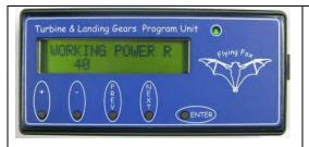
Press the "NEXT" key to enter the front landing gear (R) "working power supply" programming page "WORKING POWER R"
