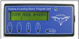
When the value is 1 it works as follows: wheel doors A + B open; gears down; wheel doors B closed – wheel doors B open; gears up; wheel doors A + B closed
