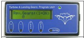
Press the "NEXT" key to enter the programming page in which it is possible setting the electric landing gears open/close direction, directly from the control unit instead of the R/C transmitter
