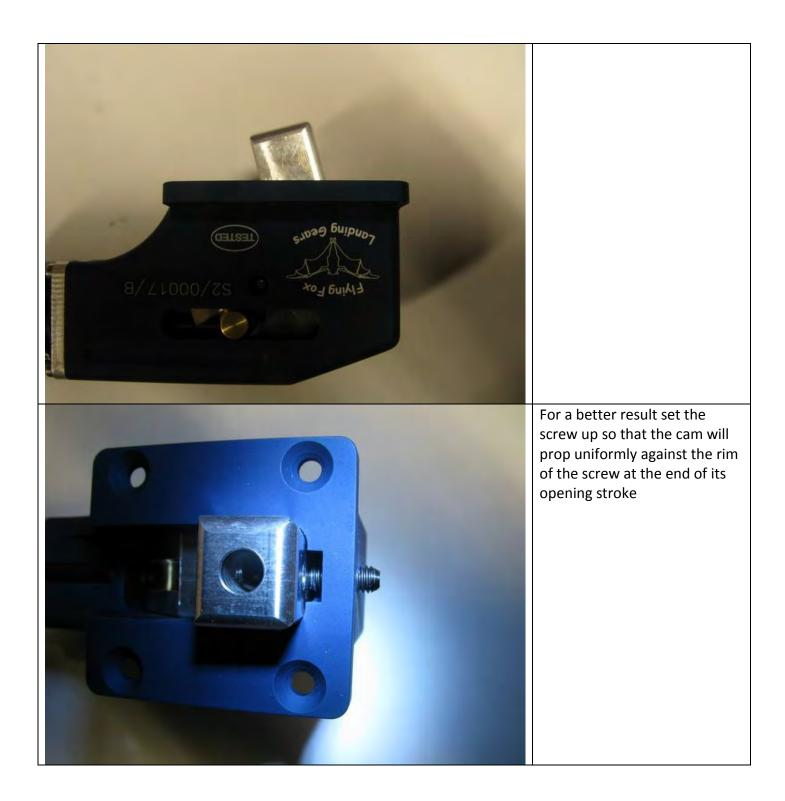
ATTENTION: to avoid the end-stroke screw screwing or unscrewing when the landing gears are closed, apply some thread-locker
