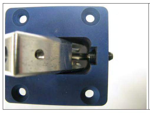
The placement of the endstroke screw in the rear part of the landing gear enables set up of the opening angle of the gear.
