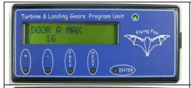
Press the "NEXT" key to enter the programming page in which it is possible to adjust the stroke value (MAX) of the wheel doors group A servos
