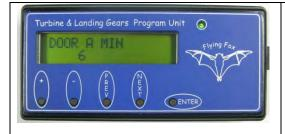
In this programming page it is possible to adjust the stroke value (MIN) of the wheel doors group A servos
