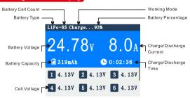
Rotating the roller wheel up or down during charging will switch the information displayed on the lower half of the LCD screen between cell voltage, cell IR and working parameters. Cell voltage and IR can only be displayed during the balance charging process.
